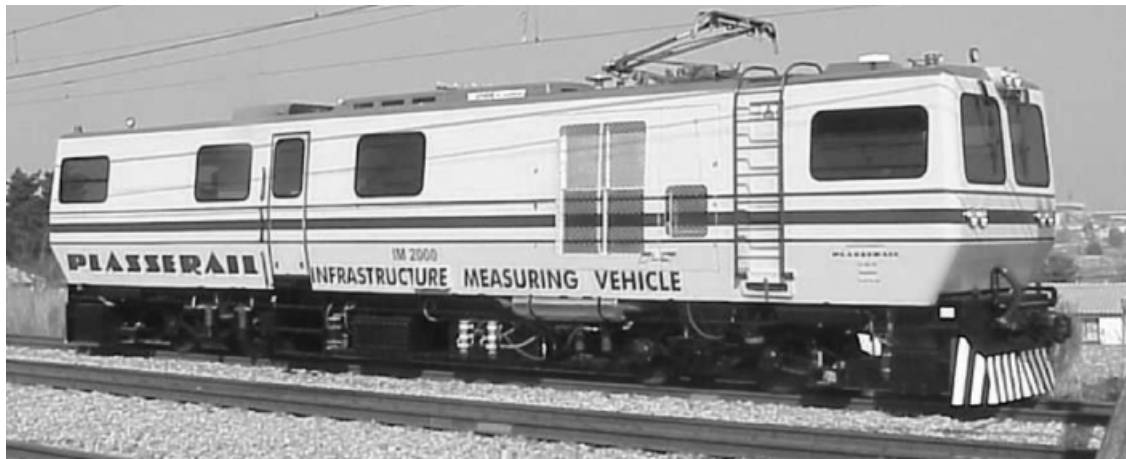
Fig. 1. The IM2000 testing vehicle used by SPOORNET to service rail tracks.
